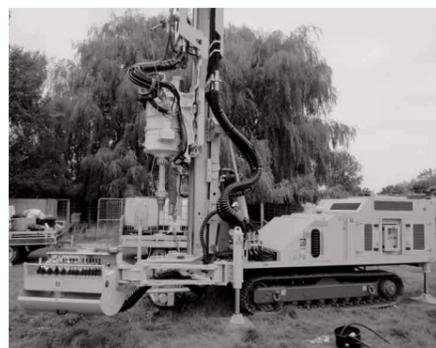
Hydraulic crawler mounted drilling rigs specifically suitable to perform drillings for the installation of borehole heat exchangers (BHE) and water well drilling. These units use all rotary and/or rotary percussive drilling systems and Down the Hole Hammer (D.T.H). Among these specific units the GEO 909 GT is the unique one with a patented automatic loading system for drilling rods and casings.
