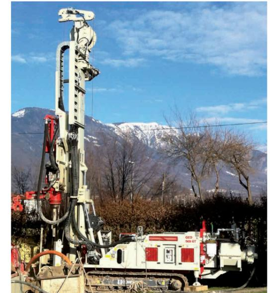
Small-medium size hydraulic drilling rig, based on the size of the GEO 601, the version called GEO 602 is equipped with a more powerful mast and a double head system able to perform:
