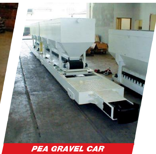
TUNNELING PEA GRAVEL CARRIER
