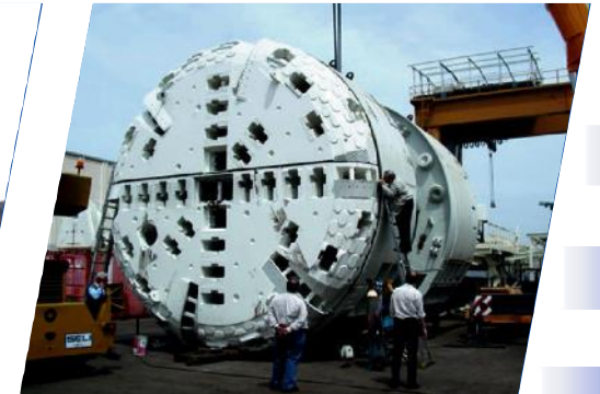
\varnothing 6980mm TBM HEAD
