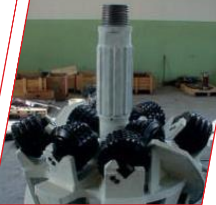
Ø 1600mm HORIZONTAL BORING HEAD
